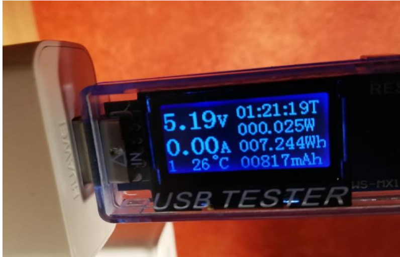
USB tester: Voltage (V) , Time, recent power (W), current (A), capacity (Wh, mAh), Temperature (°C)
